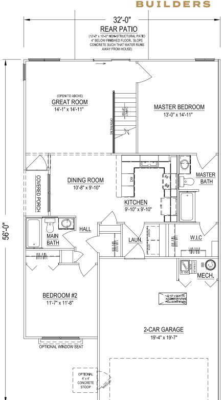
\*NOTE: 2' MAY NEED TO BE ADDED TO GARAGE DEPTH OF "B-SIDE" UNIT, IF SAME MODELS ARE CHOSEN FOR BOTH SIDES OF DUPLEX.\*
